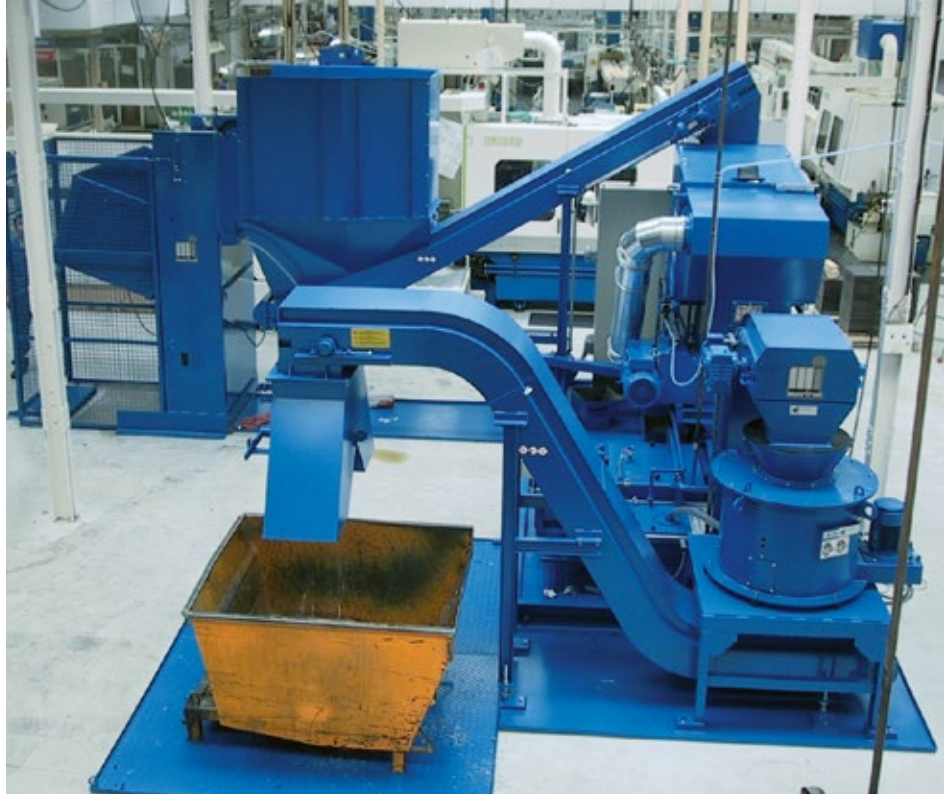
Installation consisting out of following components: swarf-wringer, swarf crusher, swarf-conveyor and container loading system.
